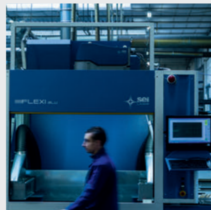
Laser micro-etching machine for PMMA.
