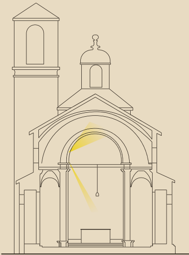
Church standard lighting | Indirect lighting + Accent lighting
