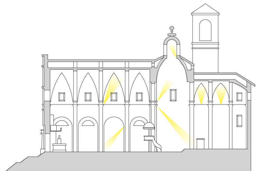
Catholic church, general lighting scheme | Longitudinal section
